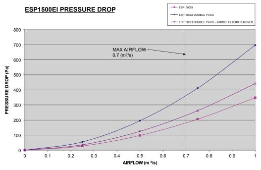
Figure 8 - Graph of ESP 1500El Pressure Drop
