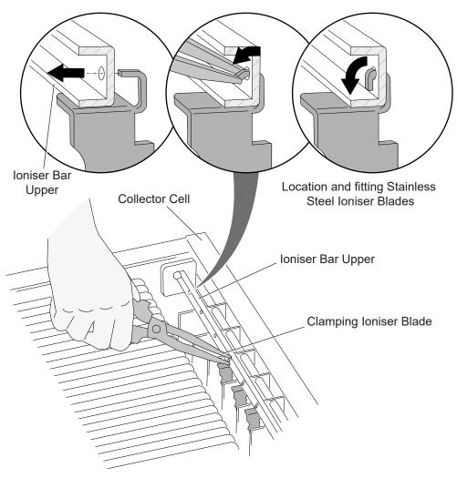
Figure 17 - Fitting Stainless Steel Ioniser Blades
