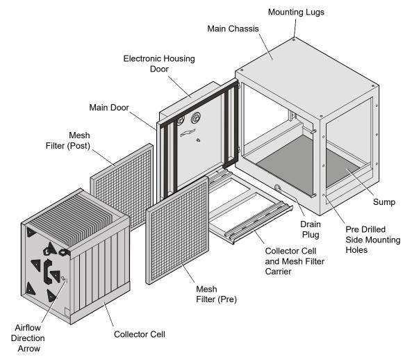
Figure 5 - Electrostatic Precipitator Unit - Main Chassis Components
