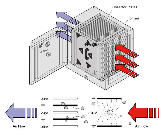
Figure 4 - Electrostatic Precipitator (ESP) - Operating Principles
