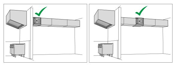
Figure 12 - Preferred Mounting of Filter Unit
