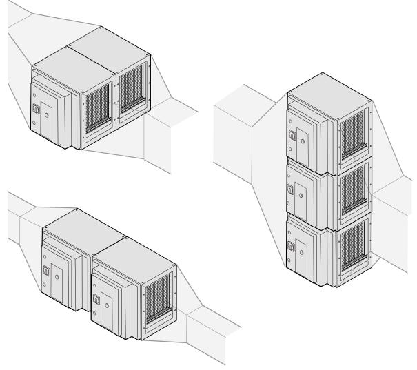
Figure 13 - Multiple Unit Installation Examples
