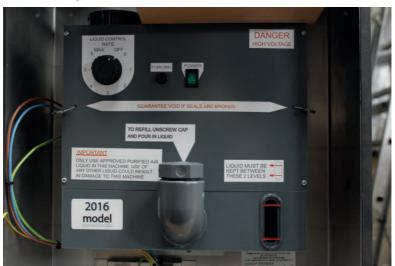
Figure 11 - Liquid Control Rate Knob and Filler Cap
