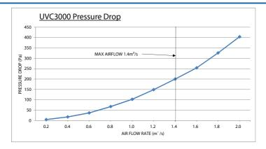
Figure 11 - Pressure Loss Graph - UV-C 3000
