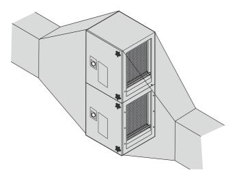
Figure 13 - UV-C 1500 Unit Installed
