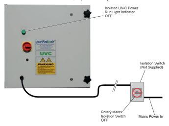
Figure 15 - UV-C with Isolation Switch
