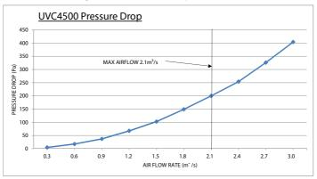
Figure 12 - Pressure Loss Graph - UV-C 4500
