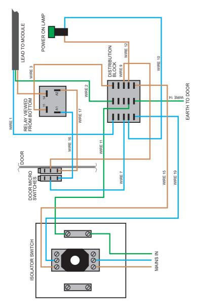
Figure 17 - Door Wiring Diagram
