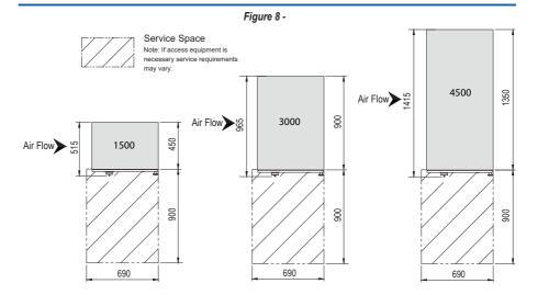
Figure 9 - UV-C 1500, UV-C 3000 and 4500 - Space Required for Accessing Light Modules
