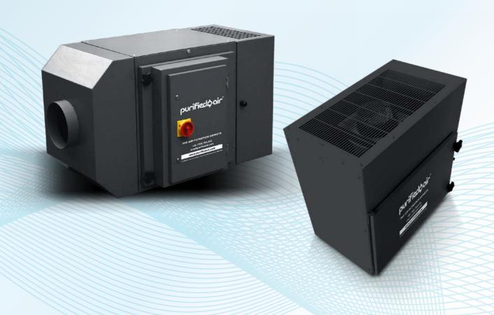
Our Oil Mist Units features a double-pass ESP technology and is efficient at 99%. Due to their compact size and built in fan system, they can be directly mounted to a machine tool. The ionisation voltage has been designed to run at a positive potential, reducing ozone production and making it ideal for indoor applications.
