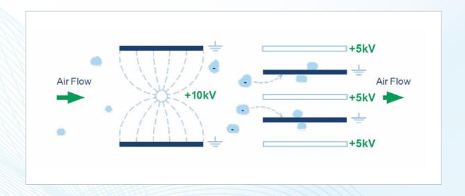
The above diagram shows, in a basic visual, how an electrostatic precipitator works:
