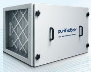
Our MFUs are designed explicitly for kitchen extract systems; they collect the oil, grease and smoke particles filtered out of the exhaust through a combination of passive air filters, including panel, bag, HEPA and carbon.
