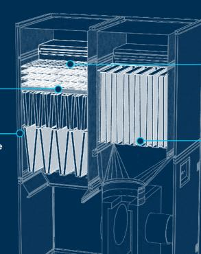
**Stainless Steel Mesh** Filters larger grease particulate.
