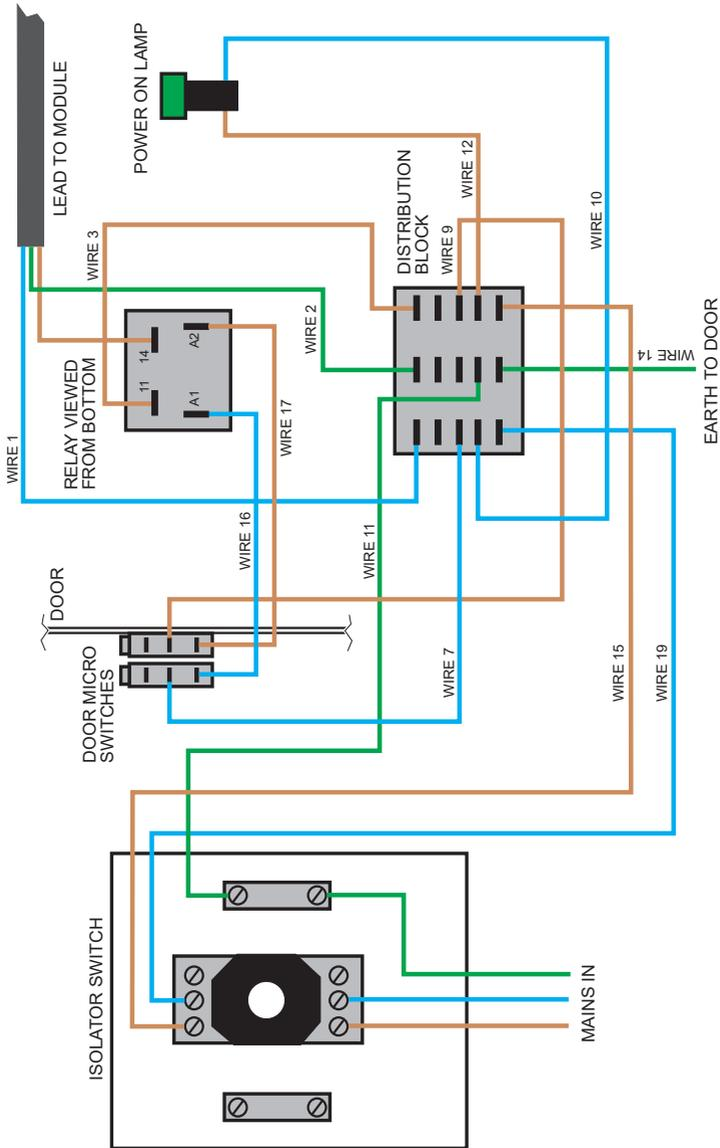
Figure 17 - Door Wiring Diagram
