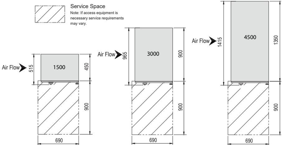
Figure 9 - UV-C 1500, UV-C 3000 and 4500 - Space Required for Accessing Light Modules
