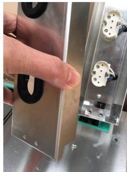
Locate the front cover into place and secure with the two Cover Screws previously removed.
