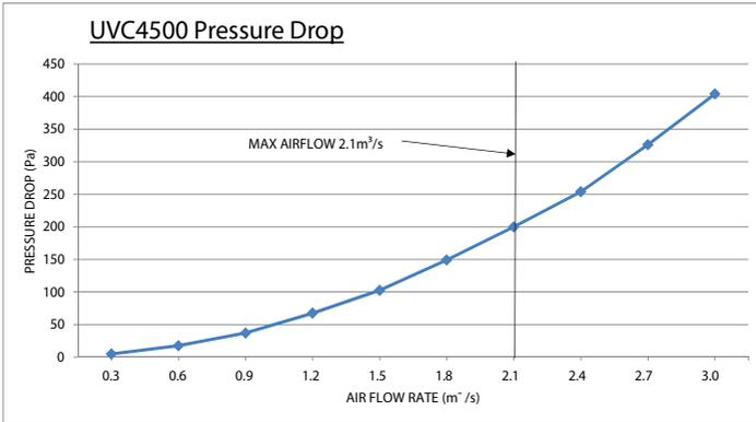
Figure 12 - Pressure Loss Graph - UV-C 4500
