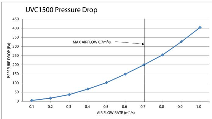
Figure 10 - Pressure Loss Graph - UV-C 1500
