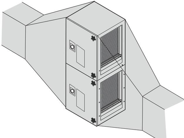
*Figure 13 - UV-C 1500 Unit Installed*
