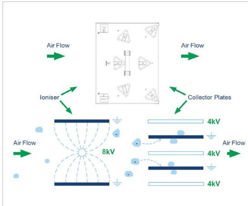
The diagram to the left shows, in a basic visual, how an electrostatic precipitator works. As air passes into the combined ioniser / collector cell, the particulates in the air stream are polarised. As they continue through the ioniser and between the collector cell plates, the polarised particulates are repelled away from the positively charged plates and attracted to the earthed plates where they stick and so are filtered out of the air flow.
